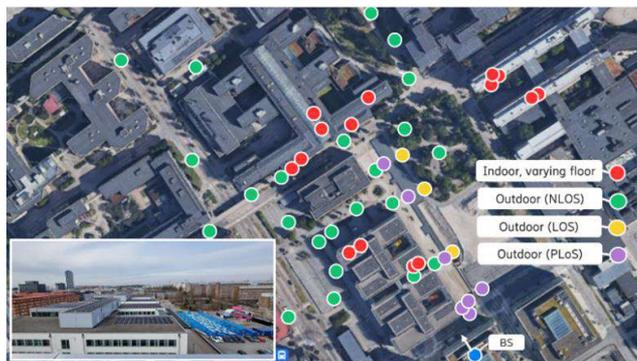
Fig. 3: Experiment scenario. Here, 46 Tx devices transmit to a BS. Channel samples were logged and analyzed, extracting LSPs.
